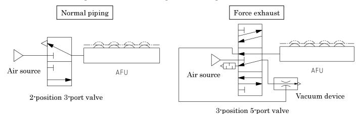
\*The Freebear part of this product does not descent naturally when air is exhausted during the downward operation, due to resistance from the cylinder's O-ring, among other factors. (Residual pressure has been released, so it will descent under the load of the transported item's own way, etc.) If it is necessary to force the Freebear part to descend,
