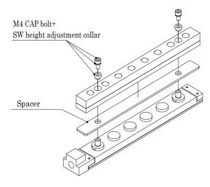
Adjust height using spacers (thickness and number) \*\*It is necessary to change the collar and bolt at the same time.
