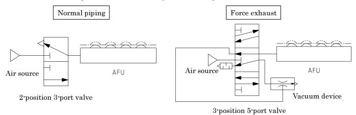
\*The Freebear part of this product does not descent naturally when air is exhausted during the downward operation, due to resistance from the cylinder's O-ring, among other factors. (Residual pressure has been released, so it will descent under the load of the transported item's own way, etc.) If it is necessary to force the Freebear part to descend, please refer to the "Forced exhaust" circuit.
