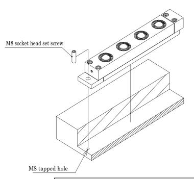
\*This product is not designed for complete fixation to the installation surface. For complete fixation, please use the AFU·3232·4P series.
