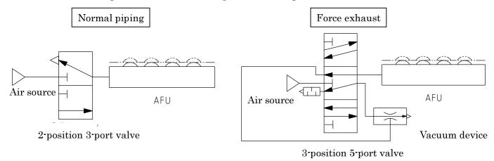
\*The Freebear part of this product does not descent naturally when air is exhausted during the downward operation, due to resistance from the cylinder's O-ring, among other factors. (Residual pressure has been released, so it will descent under the load of the transported item's own way, etc.) If it is necessary to force the Freebear part to descend, please refer to the "Forced exhaust" circuit.
