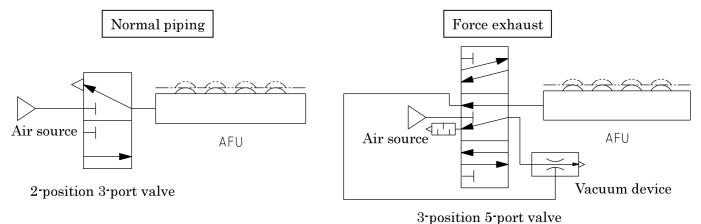
XThe Freebear part of this product does not descent naturally when air is exhausted during the downward operation, due to resistance from the cylinder's O-ring, among other factors.(Residual pressure has been released, so it will descent under the load of the transported item's own way, etc.) If it is necessary to force the Freebear part to descend, please refer to the "Forced exhaust" circuit.
